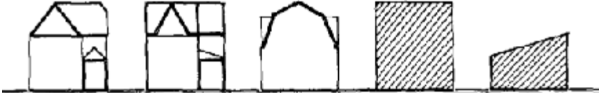
Roof shapes inconsistent with adjacent structures.
