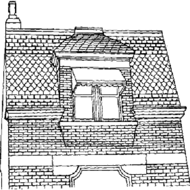
Example of an original mansard slate roof.
